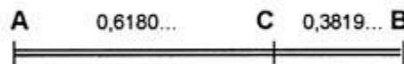
Fig. 8. Division of the segment in the extreme and middle ratio, or the Golden ratio. The segment is divided into two parts so that CB:AC = AC:AB .
